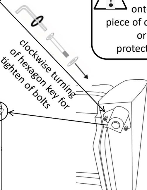
clockwise turning of hexagon key for tighten of bolts
